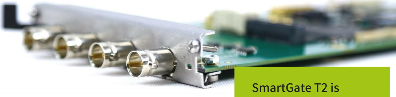
Running at the head-end, the SmartGate T2 for HDc encapsulates one or several MPEG-2 Transport Streams stemming from a DVB multiplexer into DVB-T2 BaseBand frames. It outputs the resulting T2-base or T2-lite compliant multiplex using the T2-MI (T2-Modulator Interface) protocol through ASI and IP. The SmartGate T2 runs in the HDc chassis that can embed up to 6x SmartGate T2 modules in 1U: the same chassis can output up to 6 T2-MI streams over ASI or IP.
